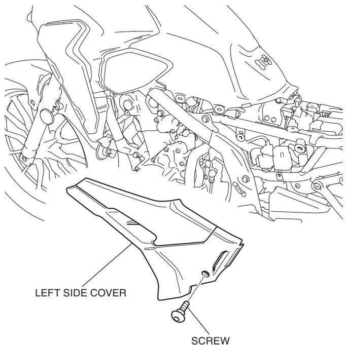
3. Remove the parts as shown.
