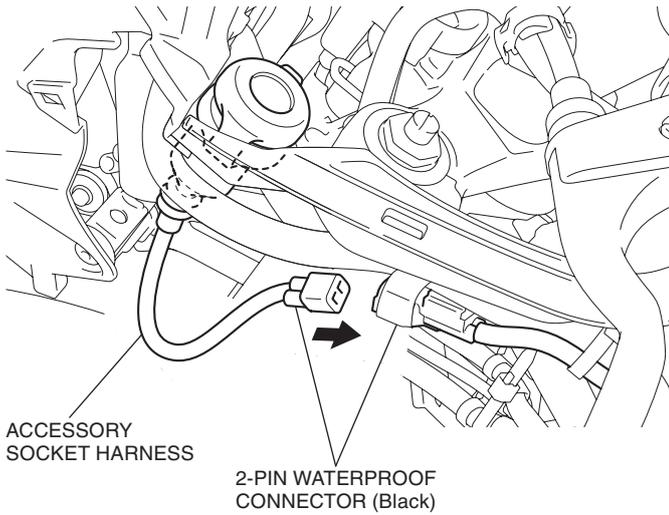
13. Secure the accessory socket harness with the wire ties as shown.
